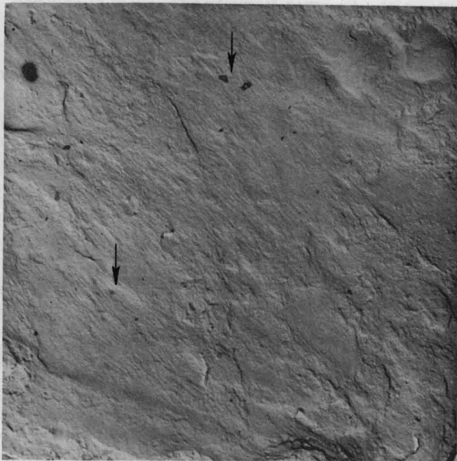
FIGURE 71. ELECTRON MICROSCOPIC FRACTOGRAPH SHOWING FINE FATIGUE STRIATIONS IN LINER OF CONTAINER I
